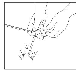
2. At the desired position, push the tent peg into the ground at an angle AWAY from the tent.
