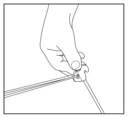
Loop guy rope through the hole in tent peg as shown above and secure.
