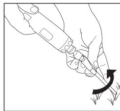
4. To remove the tent pegs after use, use a drill with the I3mm Hex head adapter provided, and set the drill to reverse.
