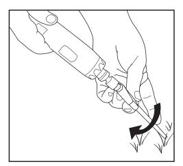
3. The tent peg can be inserted into the ground using a spanner (not included) or by using a drill with the I3mm Hex head adapter provided.
