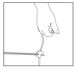
After use, pull out tent pegs using the tent peg puller supplied. Hook tent peg puller under plastic stopper.
