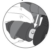
Open the Velcro strap and push the padding aside. Release the spring pressure button to subsequently pull the frame tubes apart.
