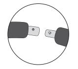
3. Make sure that a thicker tube end with a hole follows a pipe end with a spring button.
